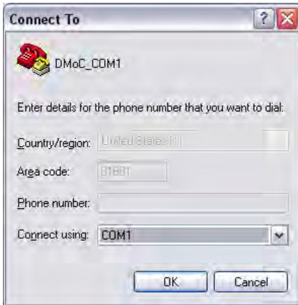
The HyperTerminal settings for communicating with the DMoC should be 19200 Baud, 8N1, with no flow control. For example, in Windows XP:
