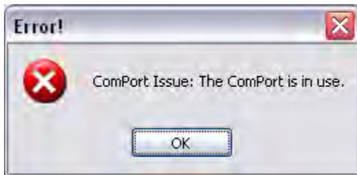
Is the COM Port being used by another application? Since ccShell thinks the ComPort is in use, be sure you closed HyperTerminal, other instances of ccShell, and any other devices using the serial port. This message should then go away. Sometimes Windows is a bit slow to release the COM port, so be patient and it might work in a few seconds. If all else fails, use the TaskManager to kill any lingering ccShell or other serial processes. Lastly, try restarting your PC.
